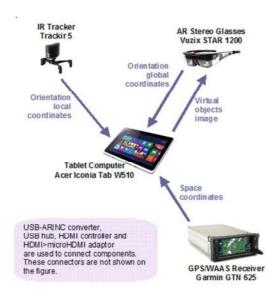
Figure 3. System architecture.
